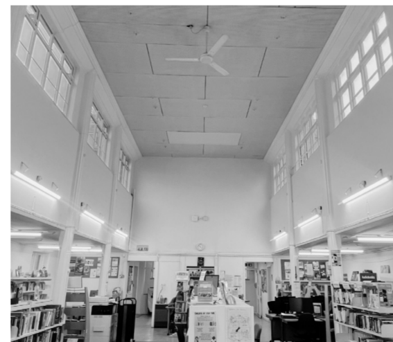
High ceiling help to create a less claustrophobic space. Windows at the top create a better illumination.
