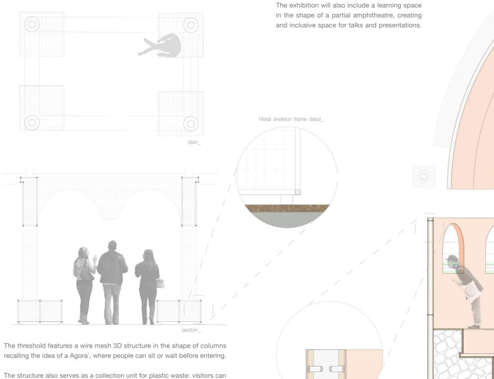
The structure also serves as a collection unit for plastic waste: visitors can dispose their recyclables by putting them through the mesh, which will than feed the 3D printer.
