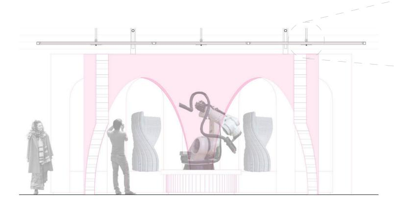
The pink room hosting the New Raw, features a 3D printing machine which will build the arched structure throughout the duration of the exhibition, utilising recycled plastic waste partially collected on site, and making it the main feature of the gallery, that will encourage people to return and witness the various stages of its creation.
