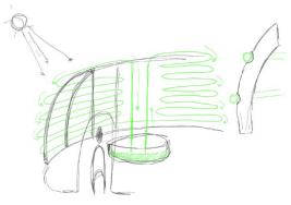
The Klarenbeek & Dros exhibition is situated in the glass house and features a real Algae Farm. This Greenhouse is comprehensive of a light wooden skeleton frame to which are anchored a series of coiled tubing that become the actual walls of the structure.
