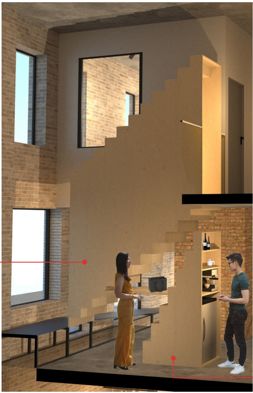
1 - Junction between an outer plywood sheet and maple tabletop 2 - Butt junction between maple "step" and "riser", which are stuck on inner plywood sheet on each side
