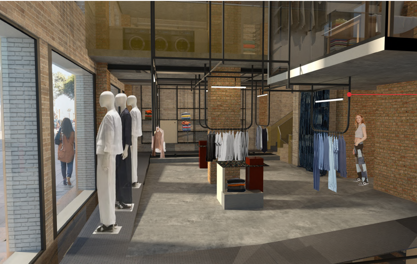
The custom hanging system, made entirely from recycled aluminium, combines sustainability with high adaptability. Suspended below different ceiling levels, a grid of horizontal tubes acts as a flexible framework for clothing racks, and integrated lighting.
