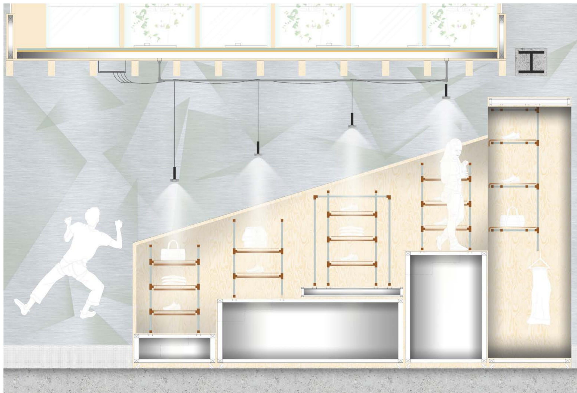
ZOOMING IN - Detail section aims to provide a clearer information of how the motion blocks are constructed, along with a closer look at the key clamp retail display. Key clamps have been chosen in order to evoke Adidas' perspective on exercise: edgy, cool & urban. Hanging lights put focus on the product. Upper Yoga space is designed with an acoustic floor in order to give maximum focus to the users of the space. Rock Climbing unit further pushes the idea of movement.
