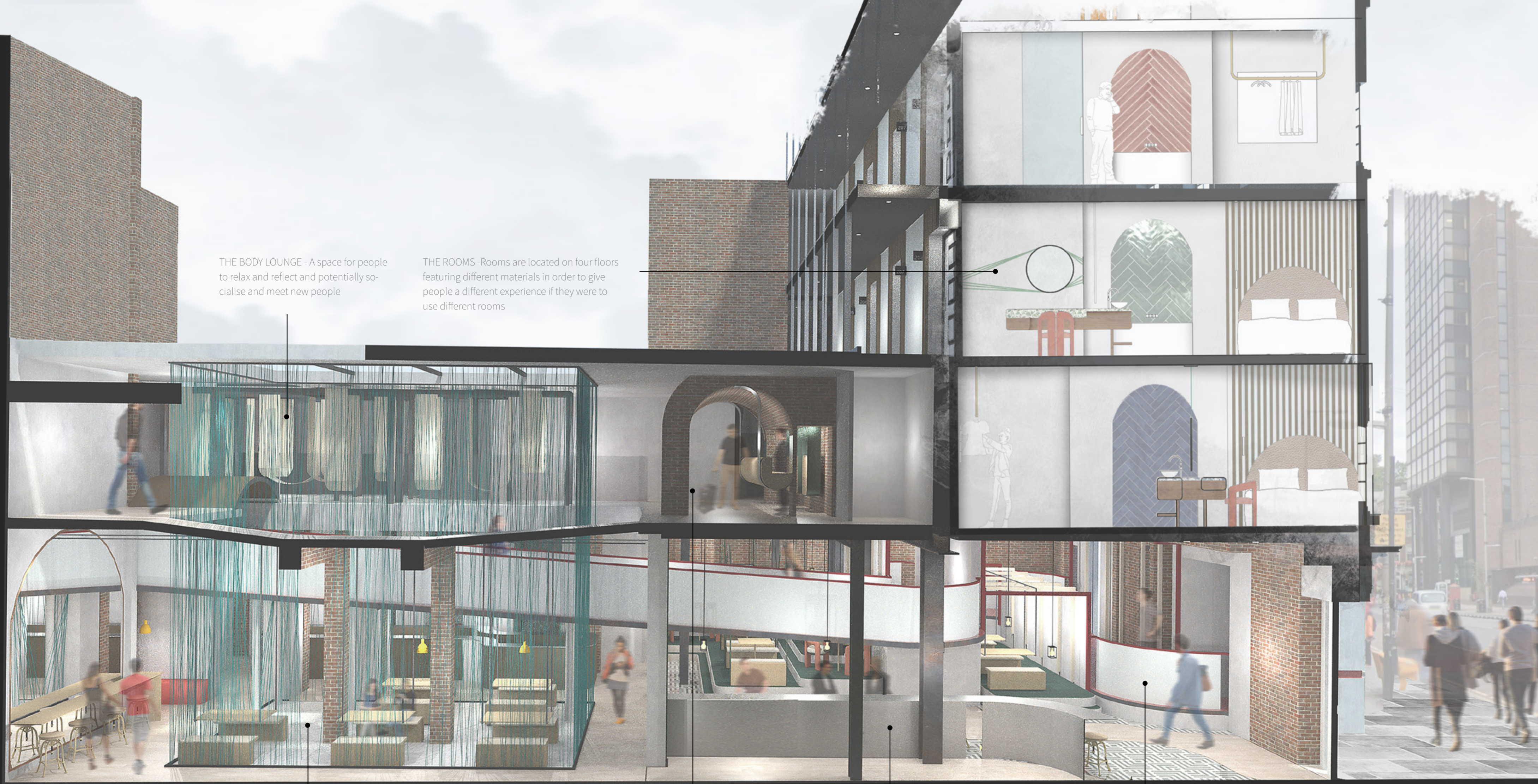
THE VOID - A space that feels as though people are outside due to the double height space and sun roof however it is located on the ground floor.
