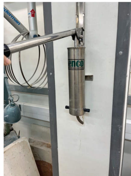
2. I added clay in this manual machine to transform it into thin round strings.
