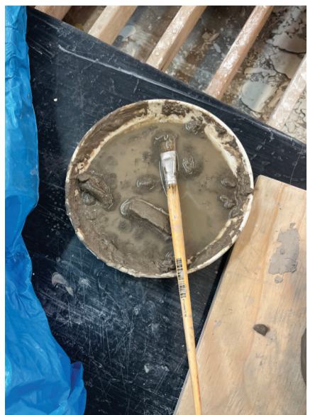
6. This is a mixture of water and dry clay. It is used to smooth the dry surfaces and make it easier to combine together.
