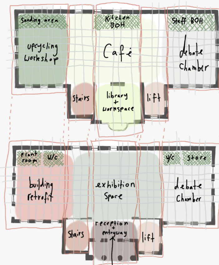
Block Plans exploring the division of space dictated by the existing building grids
