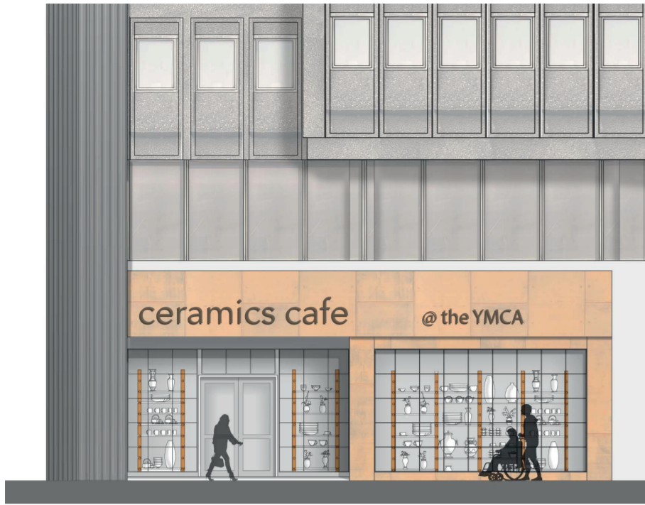
New Corten steel entrance to reflect interior language. Large display windows and entrance to encourage visitors to enter
