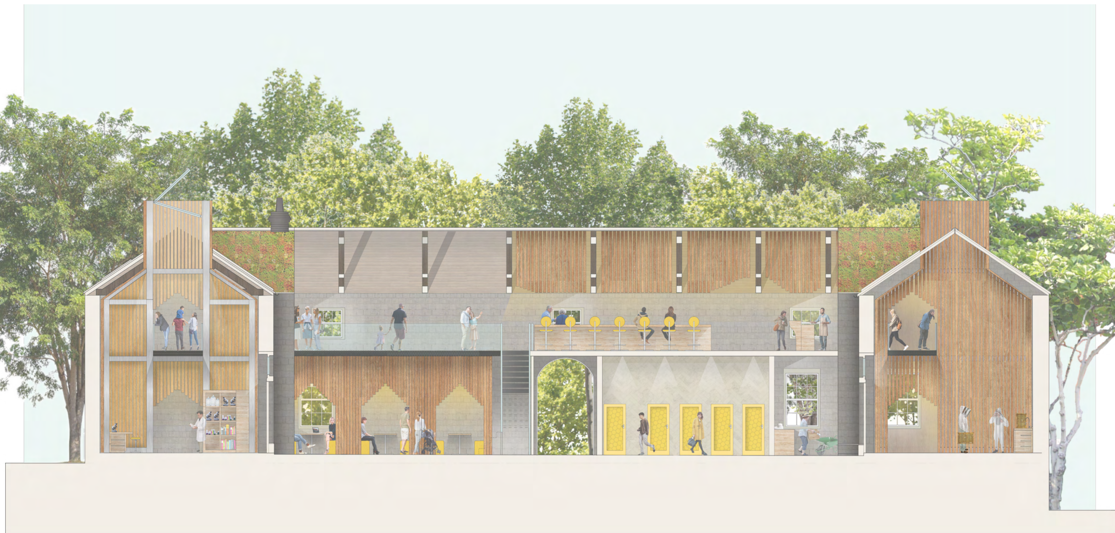
Science Lab with steel walkway above. Live beehives encased in glass located on first floor within original window opening
