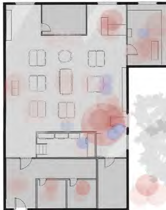
Fig. 38. Heat plan analysing the location and density of users in DRS (Newens,G.,2023).
