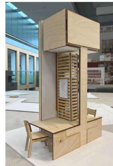
PHYSICAL SECTIONAL MODEL SCALE 1:10 SHOWING T PANEL
