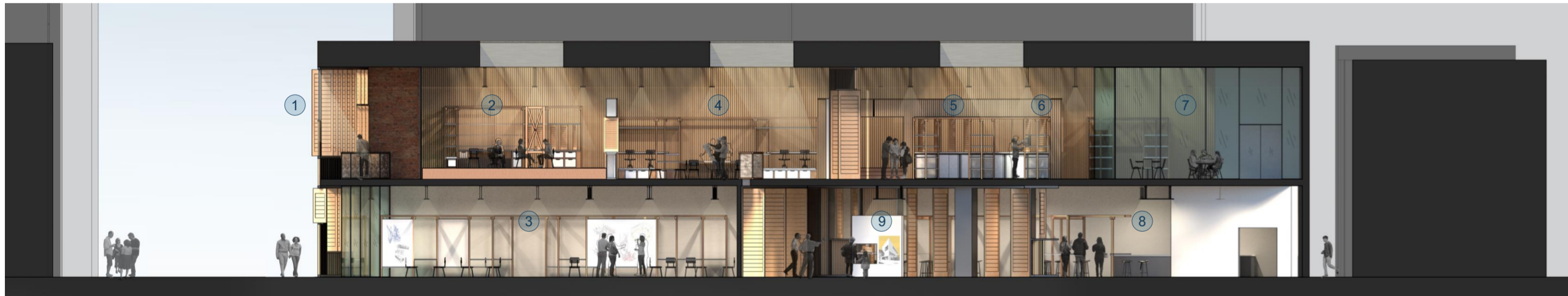
Long section drawing cutting through main functions of the Community Incubator building, including the (1) shutters wall partitions, (2) collaborative workspaces, (3) hotdesking area, (4) additional meeting/workspaces, (5) library/archive, (6) lounging space, (7) balcony, (8) cafeteria and kitchen space, (9) exhibition space.
