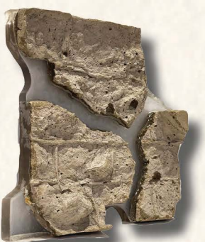
Accent wall material sample A special crafted material for Afterglow, following the concept of visible scars — made from concrete and resin
