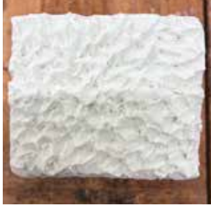
Polyethylene cut into with stanley knife to create a rocky texture
