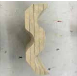
Cutting and sanding wood to develop a curved mould
