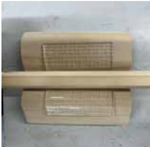
Melting acrylic onto the wooden mould and pressing down with wooden pin
