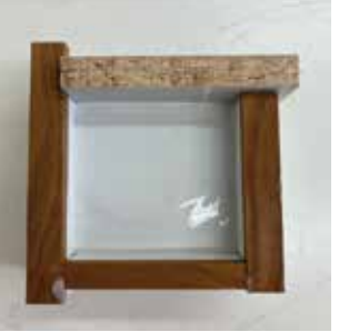
Plaster of paris mixture drying onto the polyethylene mould
