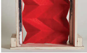
Application of felt to folding wall element shown in 1:20 model. Using paper as a structural base before applying felt and creating a pully system, allowing the felt to fold in on itself.
