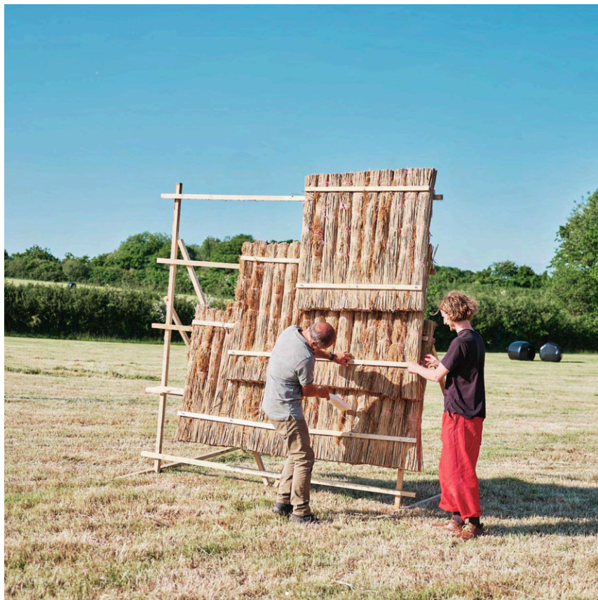
Figure 24- Testing reed cladding system, trying ways of thatching using crops from different harvests, recent instagram post (Material Cultures, 2024)
