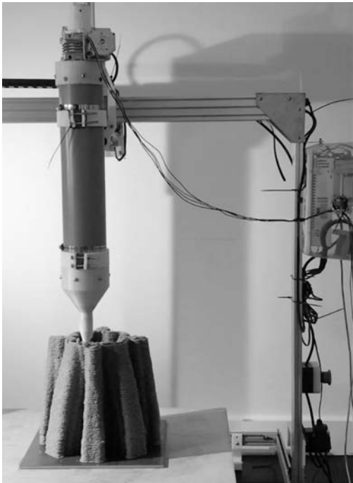
fig 2.11 3D-printed column from waste coffee cup
