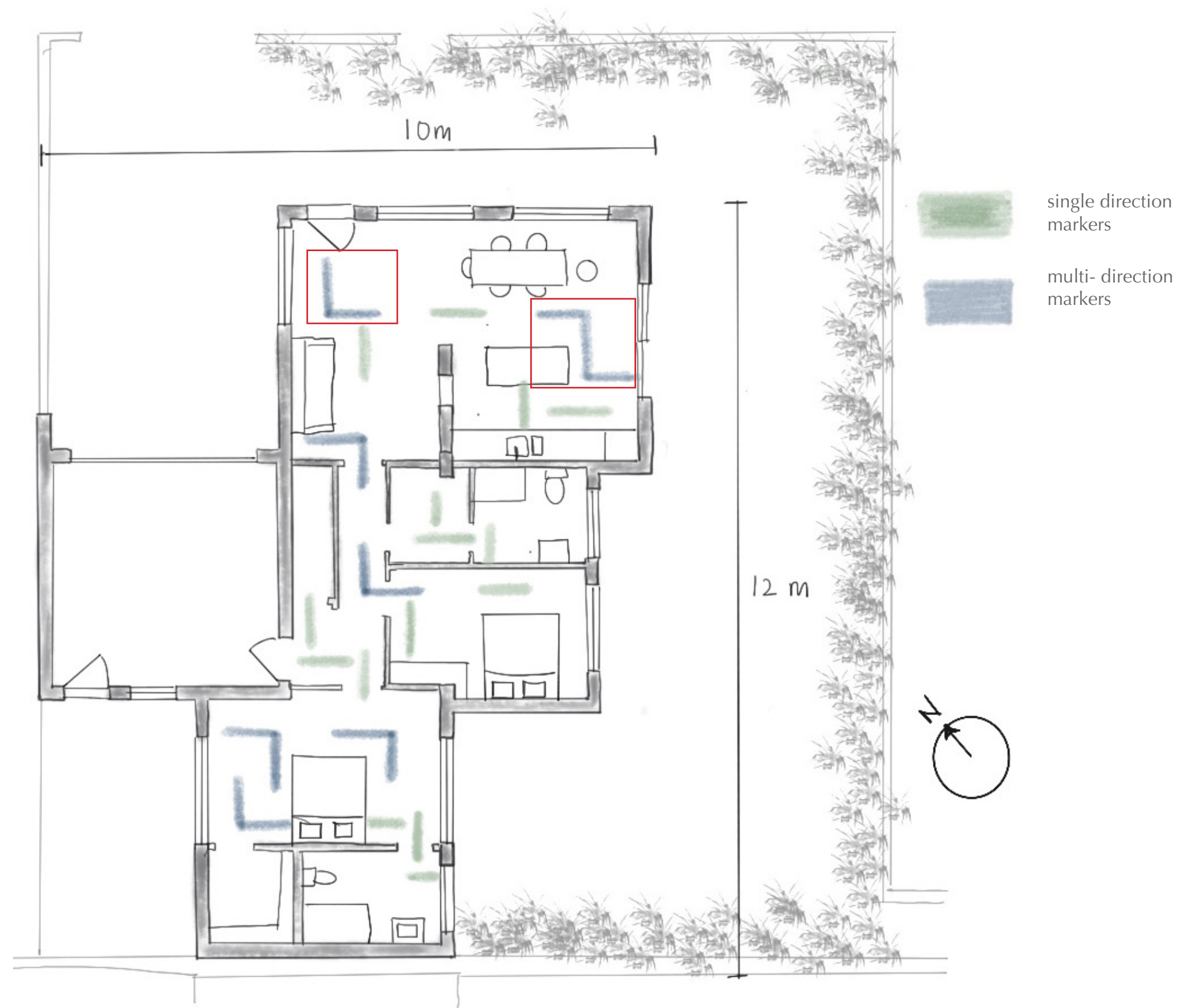
5: The patterns and cues on the floorplan of Casa Mac have been placed cleverly in rooms and junctions, to avoid accidents like bumping into furniture or the walls. The textural changes in the floor felt by the sense of touch alerts the client of obstacles. Illustration by author. 2021.
