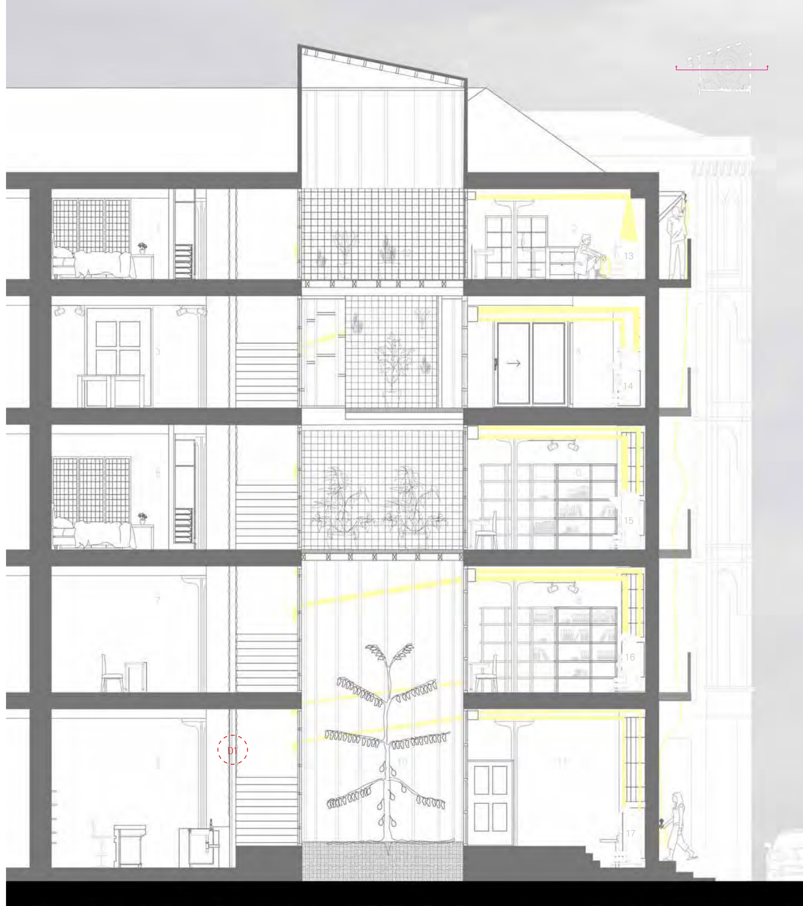
1. live-in staff accomodation 2. workshop 3. exhibition 4. archive 5. live-in staff accomodation 6. library 7. classroom/conference room 8. library 9.chocolate cafe 10. cacao farm 11. shop 12. herb's platform ●cacao chute 13. ready to process cacao bean storage 14. roasting machine 15. winnowing machine 16. grinding machine 17. conching machine
