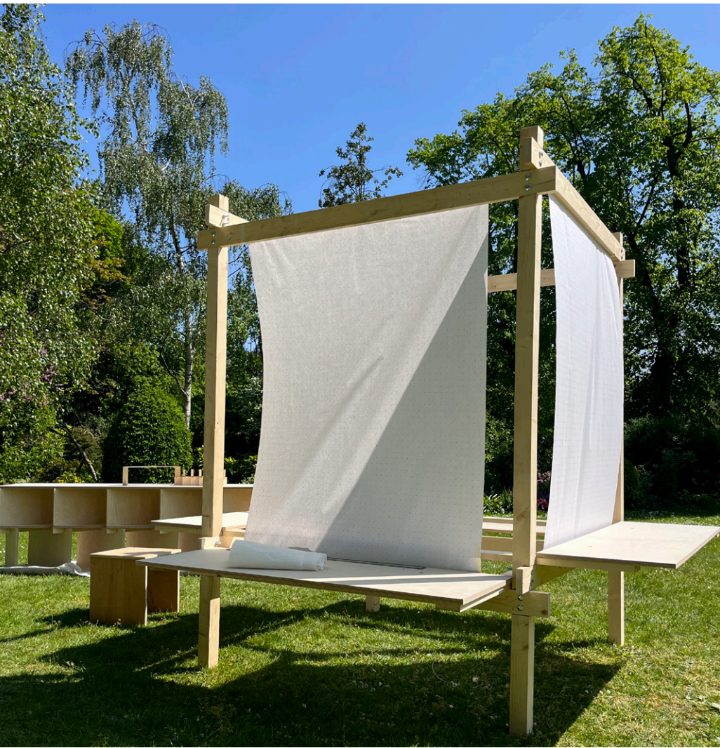
Detail 01: 1:1 installation test capturing softwood lantern assembly and model table, testing at scale allowed robust analysis and appraisal of tectonic arrangement.
