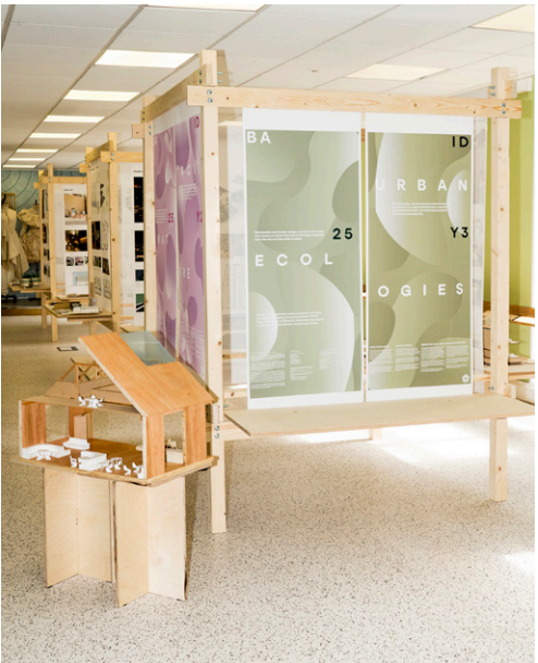
04. The exhibition tables are designed to accommodate the display of graduate large format models. Each is self supporting and demountable.
