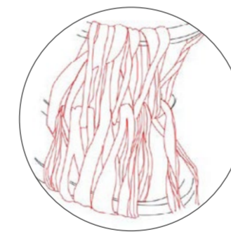
Wire and Thread Construction * Three 3mm wires will run horizontal and the yarn will be weaved between the metal wire.
