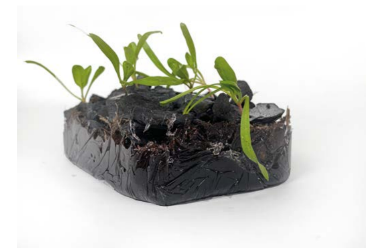
Biobrick combined within a bioplastic case as a growing medium for seeds.
