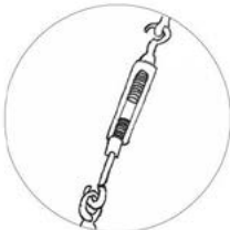
Turnbuckle This will attach to the flooring and walls to hang the suspension knitted element. Type: Hook/Hook turnbuckle
