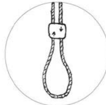
Adjustable hanging system/wire This will attach to the steel beams in the existing roofing design to suspend the knitted elements.
