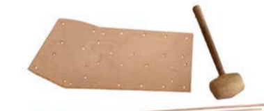
I CUT DOWN DOWN DOWEL RODS + KNOCKED THEM IN AT THE EXACT HEIGHT MODELLED IN VECTORWORKS
