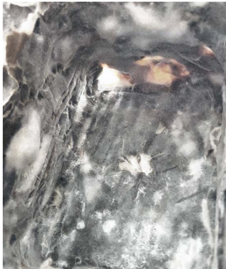
MYCELIUM REGROWTH Mycelium substrate can be pulled apart and grown on, using the same original mushroom to create more material. Growing can also be stopped by heating, so there is control over the process. Every material used in the project is strong, durable, yet able to be disposed of in a sustainable way, enriching the earth as it decomposes.
