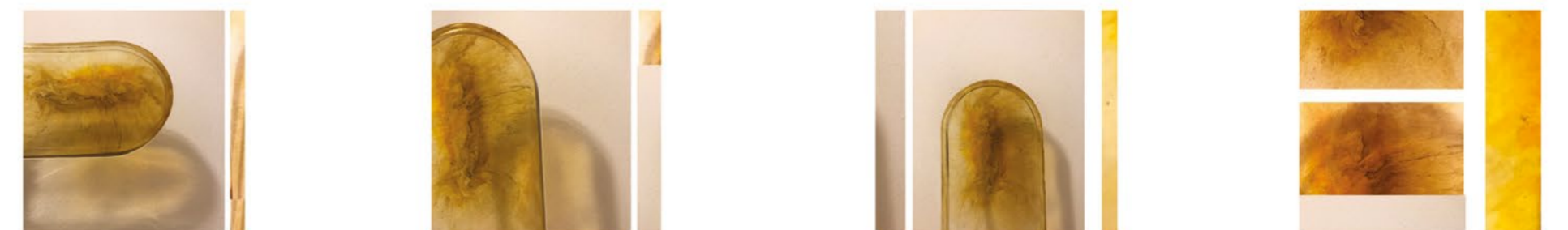
Artificial Amber made out of epoxy resin and selected resin dye to create similar look of actual Amber. The idea is to implement artificial Amber into handrail design.
