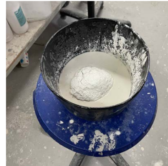
To mix the paste, I added powder water ratio and blended it. I then put the fruit in a machine which sucked all the air bubbles out of the mixture. Then poured the mixture into the cylinder with the waste in.
