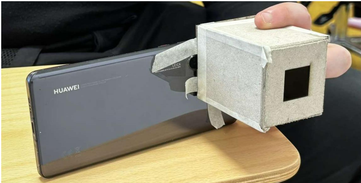
Figure 1: Camera setup for photographing conceptual lighting models for AI image input.
