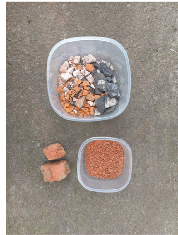
Waste materials crushed to be used in concrete mix as exposed aggregates
