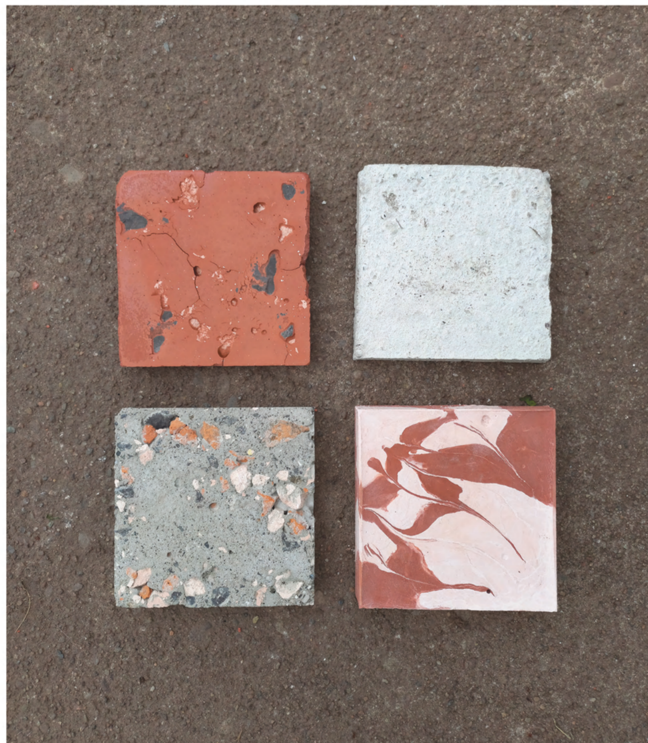
Waste materials crushed to be used in concrete mix as exposed aggregates
