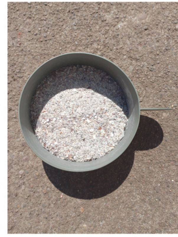
>95% Calcium Carbonate - when crushed into powder, it can be used as partial cement replacement
