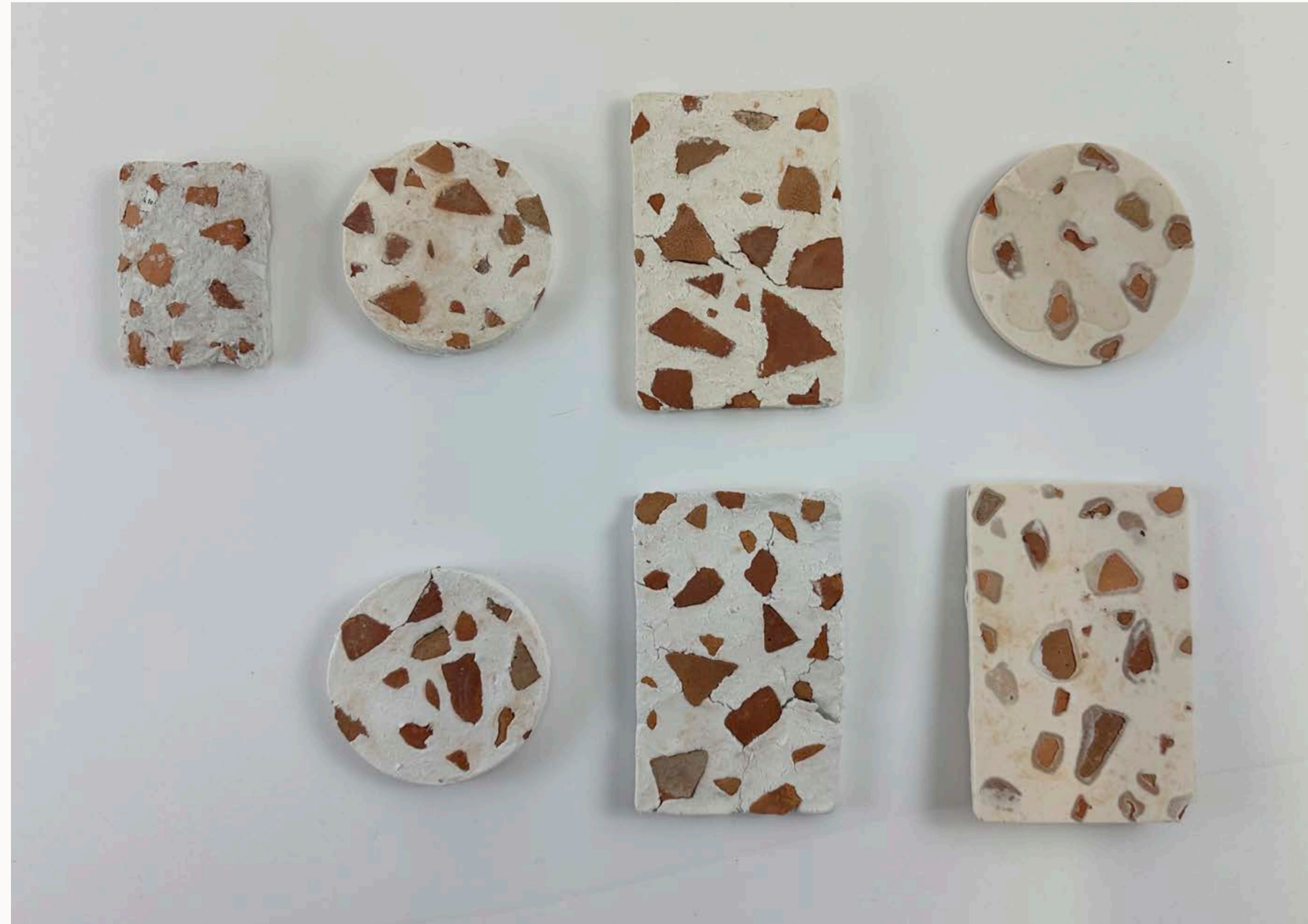
Exploration of reclaimed terracotta fragments through composite material experimentation.
