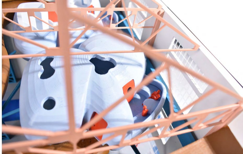
Sea view and Light control. Both pods enjoy views to the Solent through the building's existing windows and the proposed round windows on the SE façade. To avoid glare, the pods' windows have been carefully placed. Morning light from the building's NE facing roof windows come inside the pods through the pods' top windows. Their SW facing windows have been made deliberately narrow to reduce the amount of light entering the space, and easy-to-operate window treatments help controlling light
