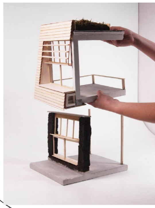
(Above) Final model showing the two primary layers of the interior. The rammed earth base is heavier with walls through which natural elements can be felt and lived within; the first floor is lighter and softly filters light, engaging with the canopy layer outside.
