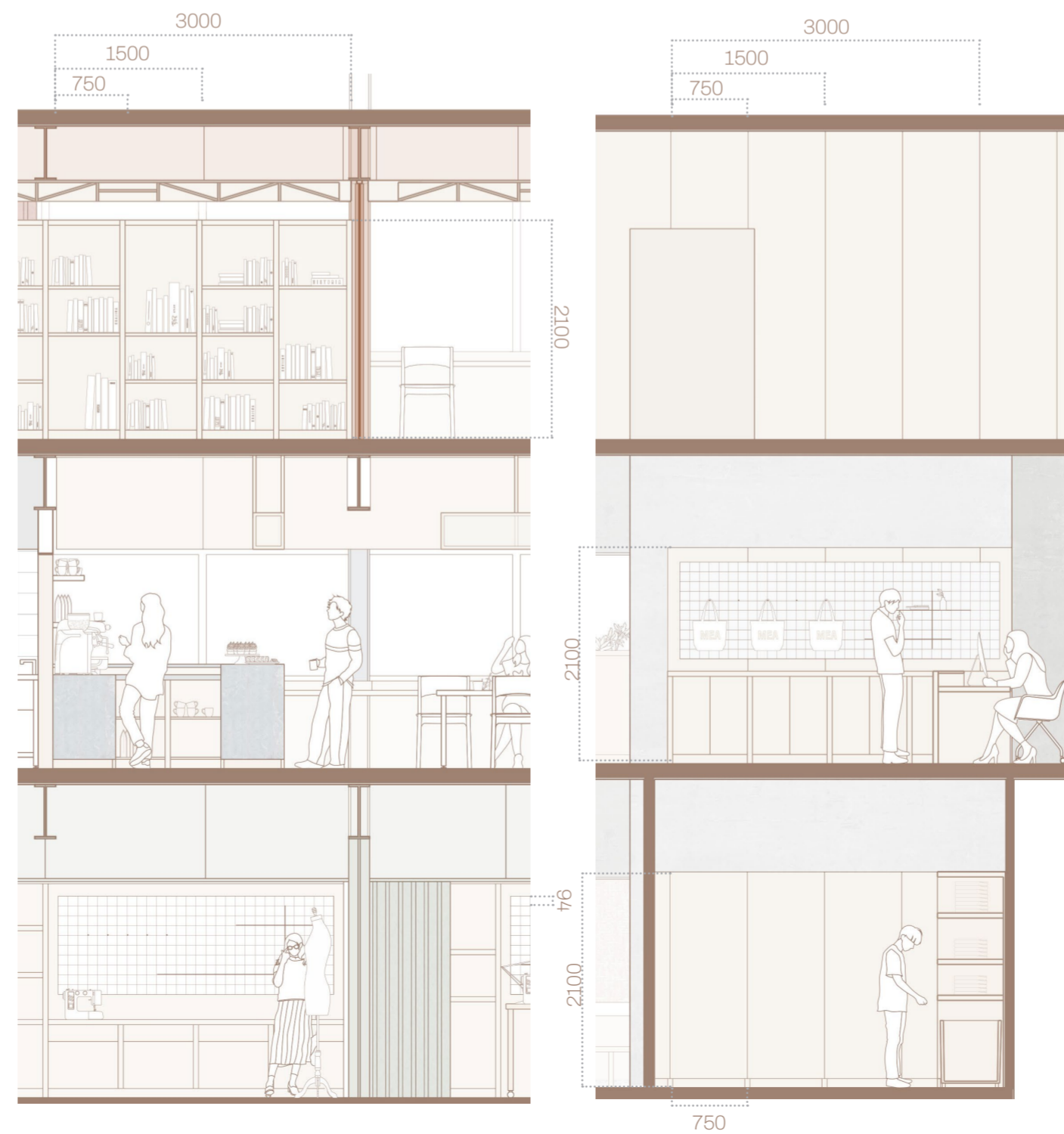
Dimensions between the balustrade railing and glazing frames, as well as the dimensions of plywood sheet correspond to the building grid. Vertical connection is created through the links in dimension, allowing spaces across floors seamlessly connect.
