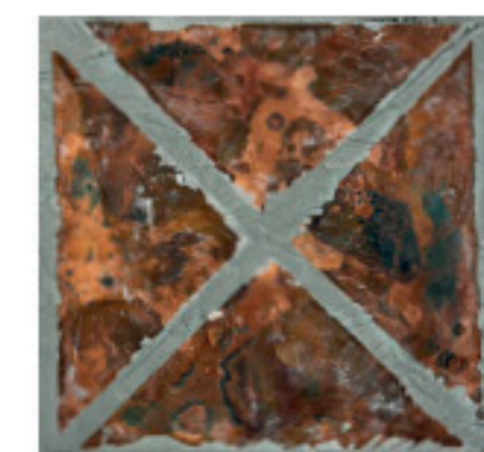
Reactivity increased with the etched surface and even created a crystallised look, mimicing the patina of copper.
