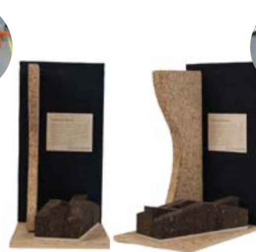
In my 1:1 sample model, cork was used as it is flexible enough to respond to the space while keeping a consistent material language.
