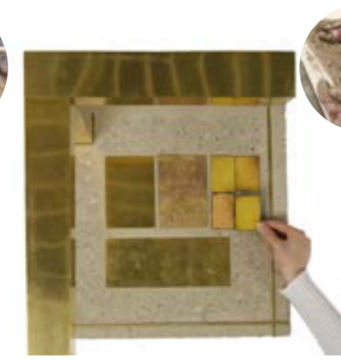
1:1 joinery prototype testing concealed dowel connections and material finishes to achieve a seamless yellow-metal aesthetic.
