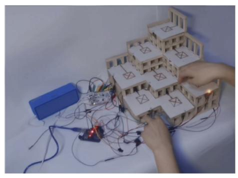
Material: Ardunio UNO board; Duinopeak Touchtouch board; Speaker; LED with 220 ohm resistor\*8; Conductive paint;
