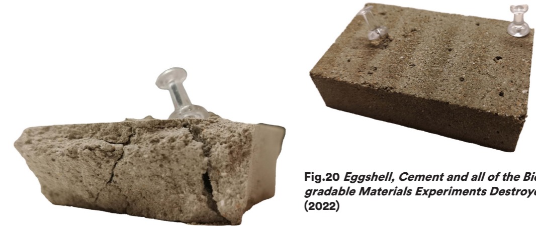
Fig.18 Eggshell , Cement and Mussel Shell Experiments Destroyed (2022)
