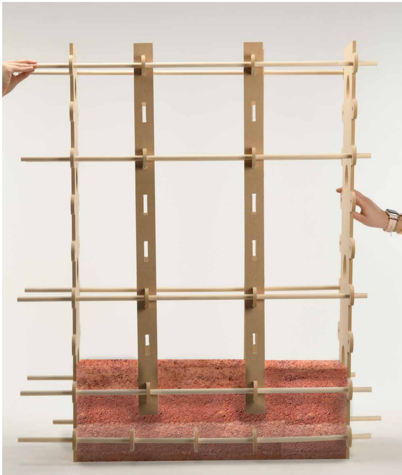
1:2 prototype with rammed earth collage
