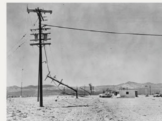
Images illustrate the wood frame house (top image) exposed to nuclear explosion with the peak overpressure 5 psi (middle) and 1.7 psi (bottom). Last image shows the collapse of utility poles on line (5psi peak overpressure) Nevada test site.
