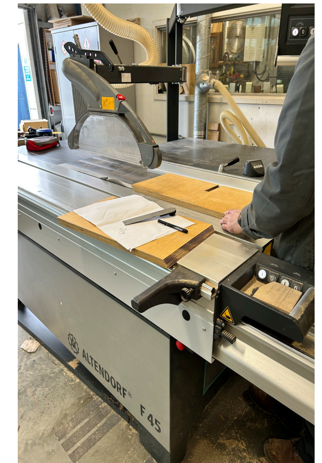
Measured and cut the upcycled door to the right size and angle needed to make the table legs using a halved joint to form the cross.
