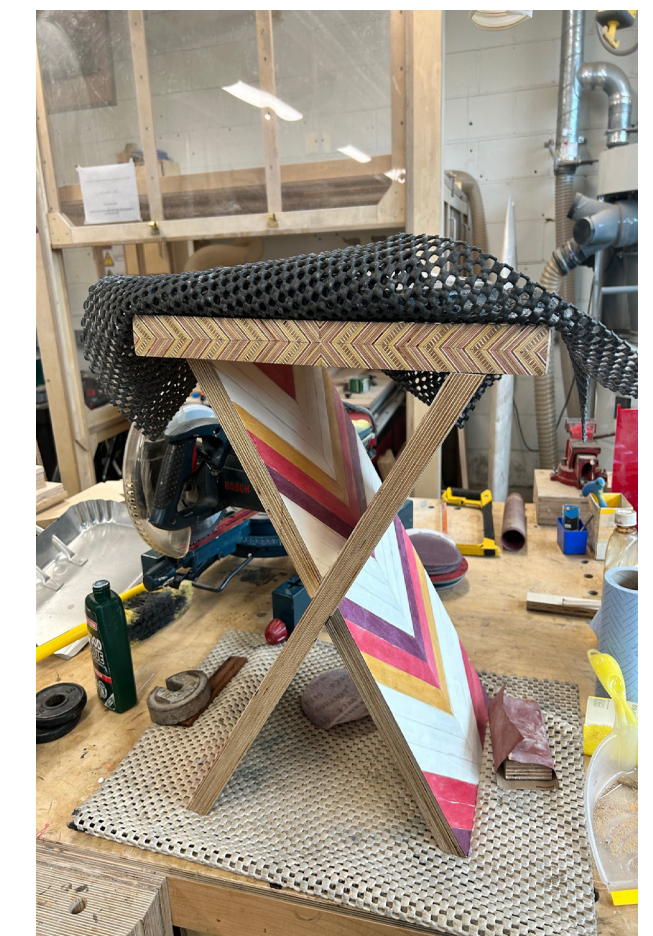
Drilled holes to the top to join the table legs to the tabletop using a dowel joint and use glue and weight to hold it together.
