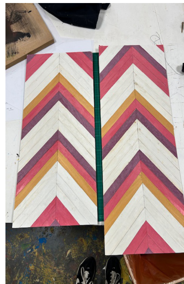
Add wood colored veneers on the outside of the legs and glue them down. To help flatten the pattern, iron it downward.
