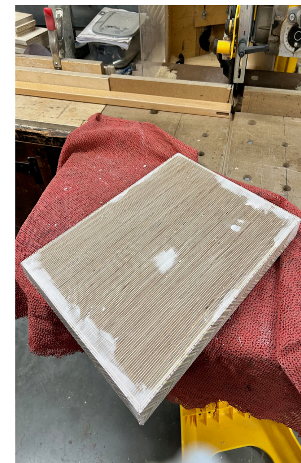
Measured and cut the plinth to work with the strips of layered plywood using a biscuit joint, then glue and fill in any gaps.
