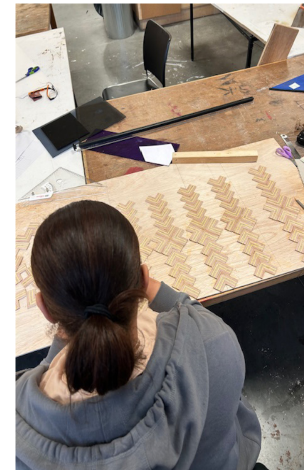
Cut the pattern block into 45° angles and create the pattern for the side of the table.
