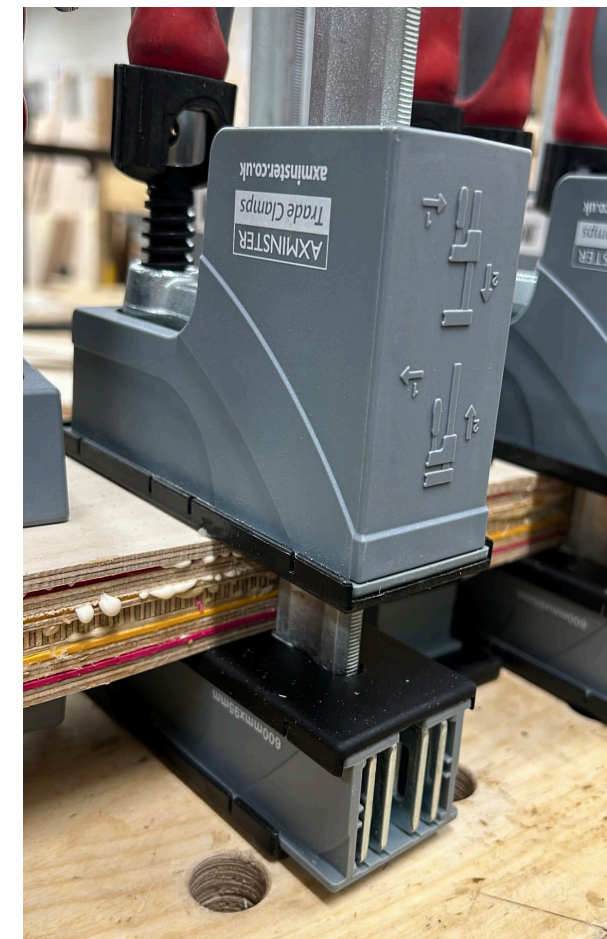
Glue all the layers of wood together using wood glue, and use clamps to help bond the elements together.
