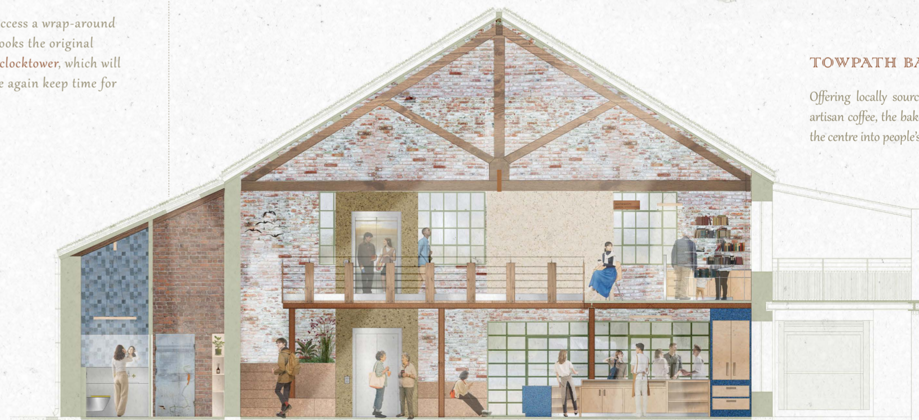
Rendered section of the Towpath Bakehouse showing main entrance point and mezzanine access.
