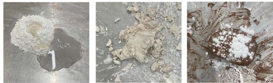
Lime based binder + Casein glue Rolling into dough-like material Adding Pigment
