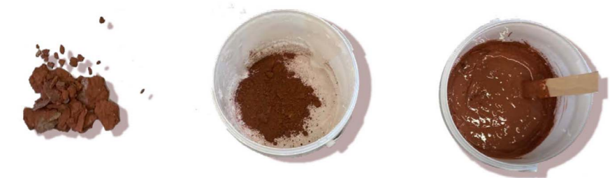
Crushing the brick Making a fine powder Mixing into binder
