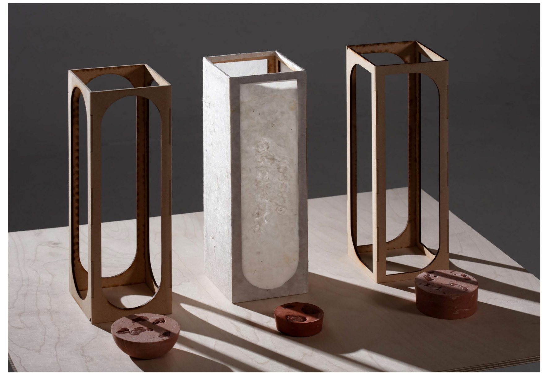
Experimenting with paper making, different thicknesses were developed to understand levels of light transmission and refine the desired atmospheric quality for the interior feature.
