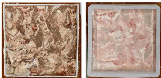
Lime based binder + Casein glue Rolling into dough-like material Adding Pigment
