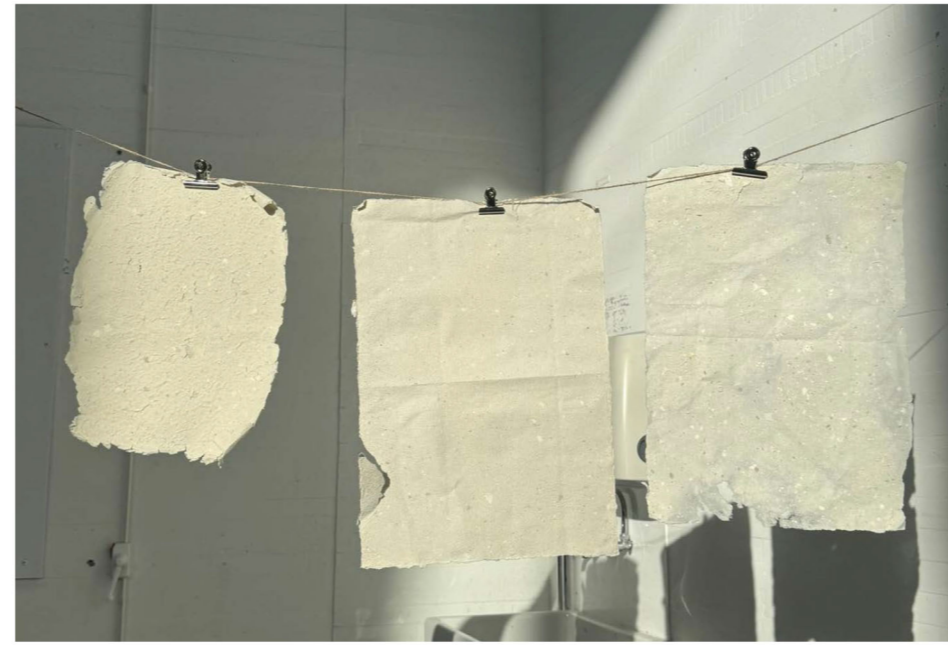
Experimenting with paper making, different thicknesses were developed to understand levels of light transmission and refine the desired atmospheric quality for the interior feature.
