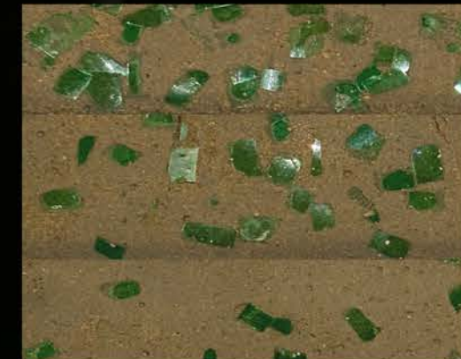
Concrete tests using plastic to reflect light with different ratios in each block.
