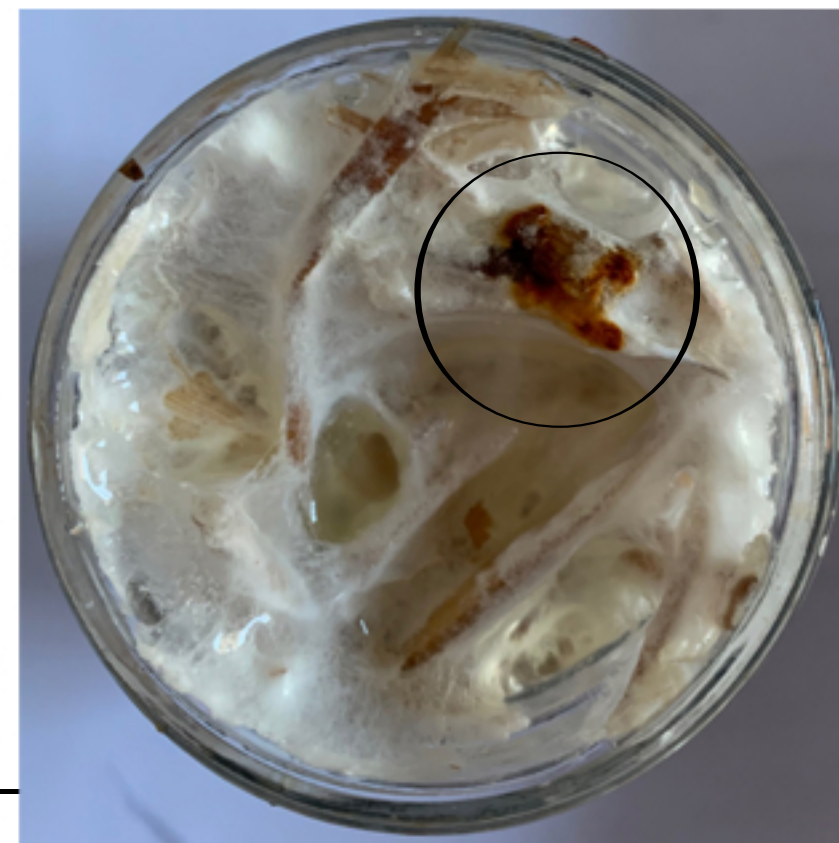
Orange mark is the Mycelium reaching the hole drilled into the lid.
