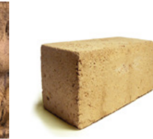
TIMBERCRETE Use: walls in staff rooms, compost, water tank, delivery area
