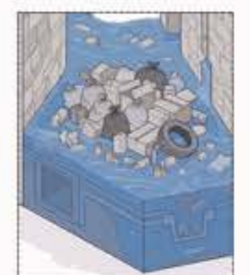
Failure (Broad Street) • Street blocks drain, causing flooding.
